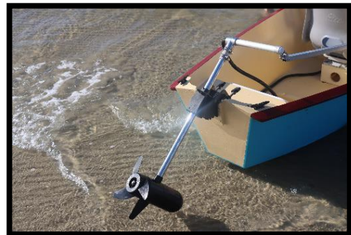
The electric drive leg, pushrod and steering arm
