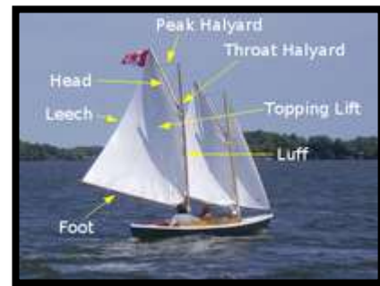
Halyards (and edges) on a gaff rigged sail
